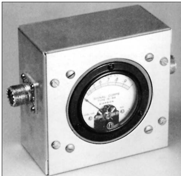
Fig 2—A convenient method of mounting an RF ammeter for use in a coaxial line. This is a metal-case instrument mounted on a thin bakelite panel. The cutout in the metal clears the edge of the meter by about \frac{1}{8} inch.
