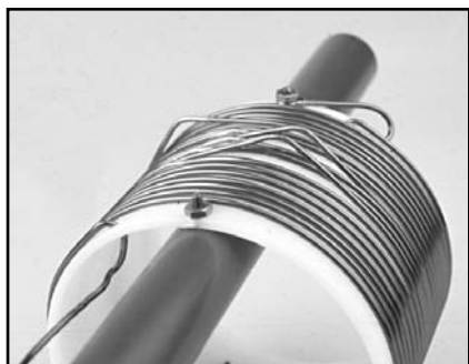
Fig 10 —Top photo shows the loading coil for the 20, 30, and 40-meter band coverage. The short aluminum tube on the coil slides into the flagpole bracket, and the tubing element slides into the other end of the PVC pipe. The wire and clip connect the element to the coil. Bottom photo shows the coil for operating the antenna on 80 meters. This is placed in the flagpole bracket and the 40-meter aluminum coil plus the tubing element is inserted into it.
