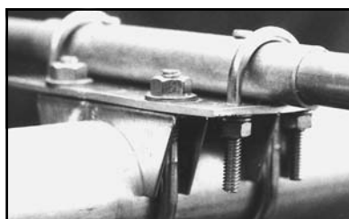
Fig 35—The element to boom clamp. U bolts are used to hold the element to the plate, and 2-in. galvanized muffler clamps hold the plates to the boom.
