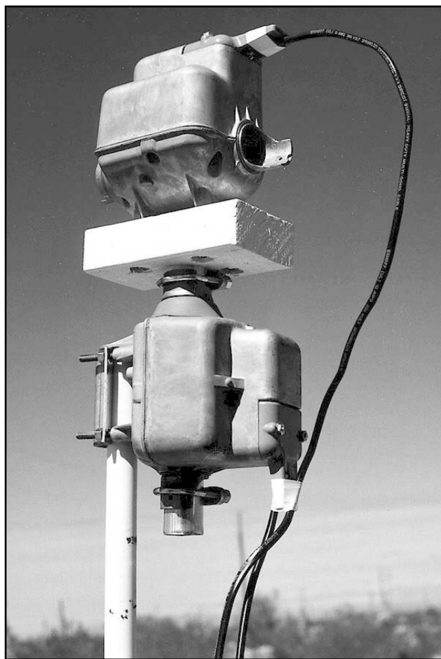
Fig 65—At left, Yaesu Az-El antenna-rotator mounting system is shown. Note that antenna loads must be more carefully balanced on this rotator than in the previously shown systems. At right, VE5FP has a solution for his Az-El rotators by bolting two of them together in his "An Inexpensive Az-El Rotator System", QST, December 1998.
