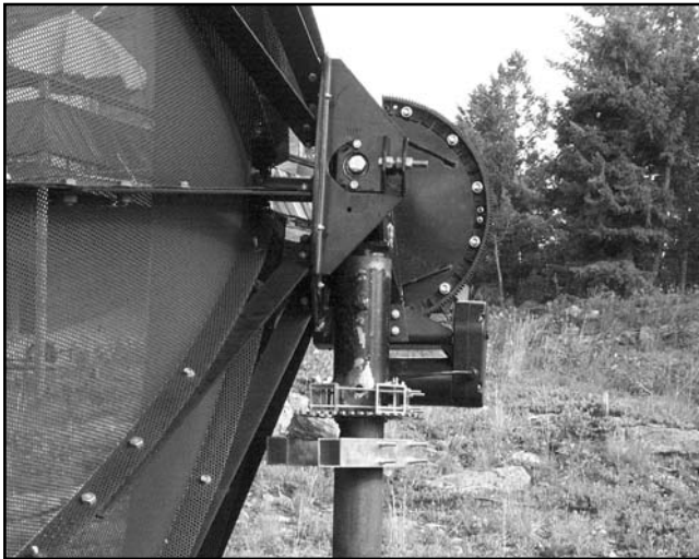
Fig 67—A modified TVRO dish mount is shown using an Az-El mount and a sector-gear drive for the elevation. (W0LMD photo.)
