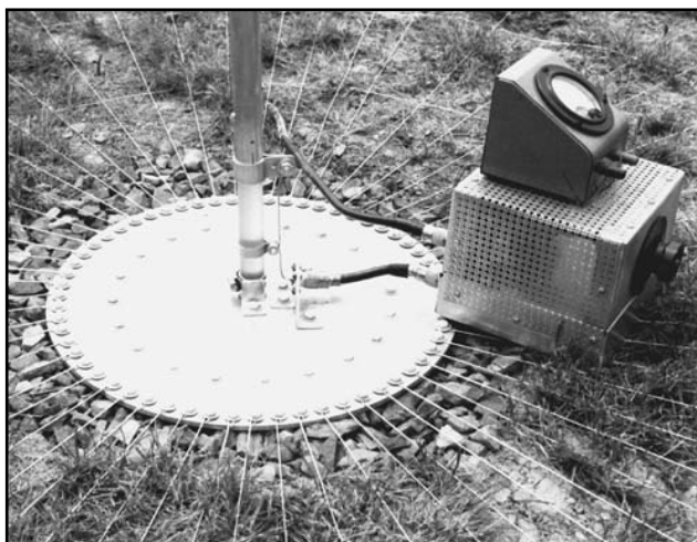
Fig 67—Base of the vertical antenna showing the 60 radial wires. The aluminum disc is 15 inches in diameter and ¼ inches thick. Sixty tapped holes for ¼-20 aluminum hex-head bolts form the outer ring and 20 form the inner ring. The inner bolts were used for performance comparisons with more than 60 radials. The insulator is polystyrene material (phenolic or Plexiglas suitable) with a 1-inch diameter. Also shown is the impedance bridge used for measuring input resistance.
