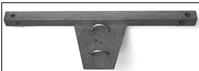
Fig 21 —Photo of the two-element quad's boom, with the plywood boom-to-mast bracket secured with wood screws and glue.
