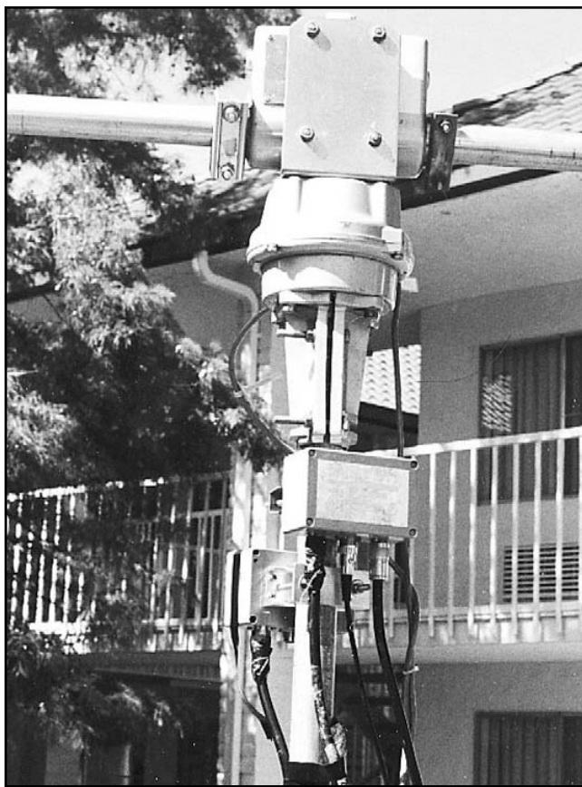
Fig 65—At left, Yaesu Az-El antenna-rotator mounting system is shown. Note that antenna loads must be more carefully balanced on this rotator than in the previously shown systems. At right, VE5FP has a solution for his Az-El rotators by bolting two of them together in his "An Inexpensive Az-El Rotator System", QST, December 1998.
