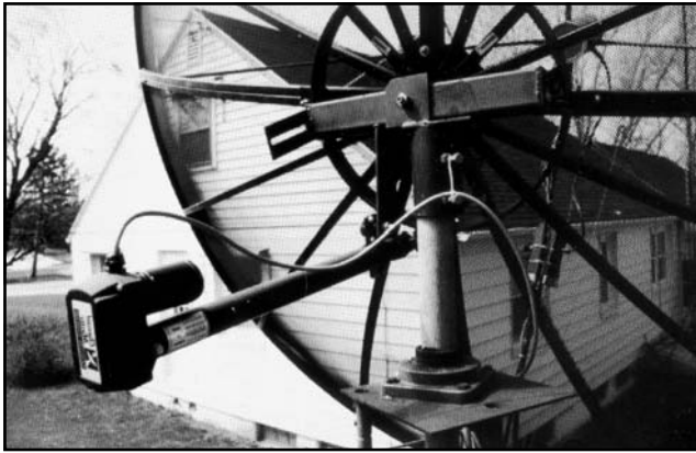
Fig 90—Elevation system, showing modified TVRO mount.
