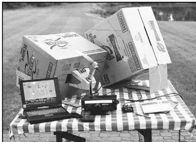
Fig 32 —A complete satellite station with the tracking laptop, FT-847 transceiver, and both downlink and uplink cardboard-box antennas.
