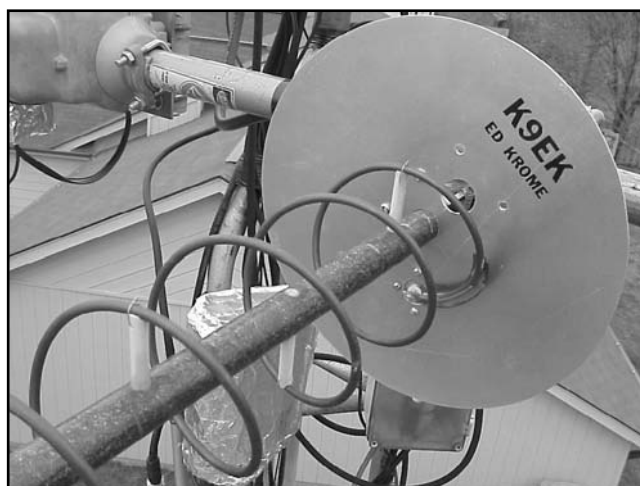
Fig 59 —At top, the method of reinforcing the reflector screen with aluminum channel stock is shown. In this version of the antenna, the three angle brackets of Fig 58 have been replaced with a surplus aluminum flange assembly. (W0CY photo.) At bottom, this helix view shows the details of a \frac{1}{4} -turn matching transformer, as discussed in the text. (K9EK photo.)
