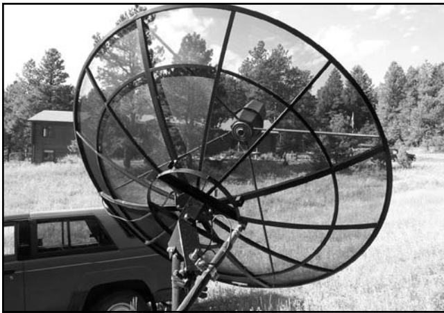
Fig 66—A TVRO dish-drive system is shown on its polar mount, using a protected drive-screw mechanism. (W0LMD photo.)
