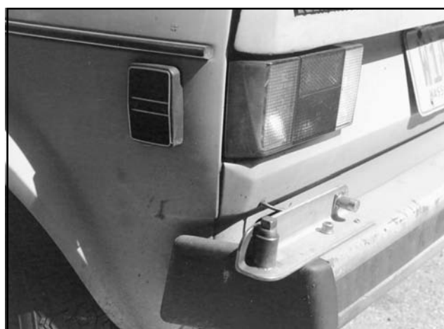
Fig 36—The mount for the mobile J is made from stainless-steel angle stock and secured to the bumper with stainless-steel hardware. Note the \frac{1}{2} -inch pipe plug and a PL-259 (with a copper disc soldered in its unthreaded end). These protect the mount and connector threads when the antenna is not in use.
