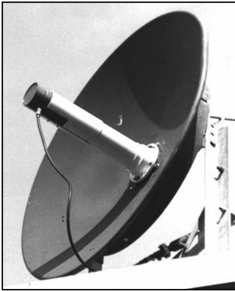
Fig 27 —Coffee-can 2304 MHz feed described in text and Fig 26 mounted on a 4-ft dish.
