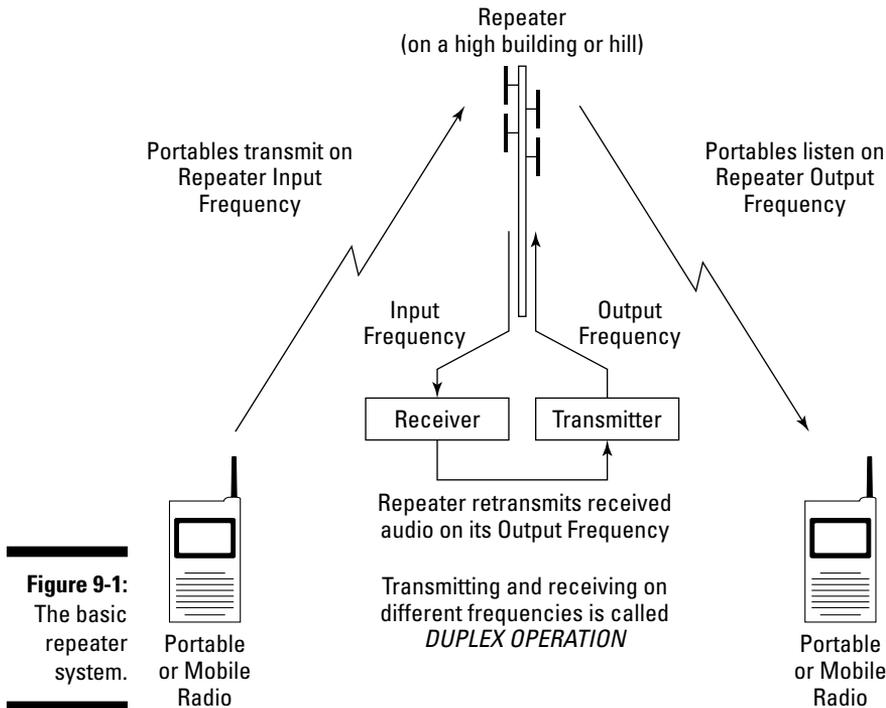
To make repeater communications work, you have to know the frequency on which a repeater listens and where it is transmitting. The listening frequency (the one that listens for your signal) is called the repeater's *input* frequency and the frequency that you listen to is called the repeater's *output* frequency. The difference between the two frequencies is called the repeater's *separation* or *offset*. The combination of a repeater's input and output frequencies is called a *repeater pair*.
