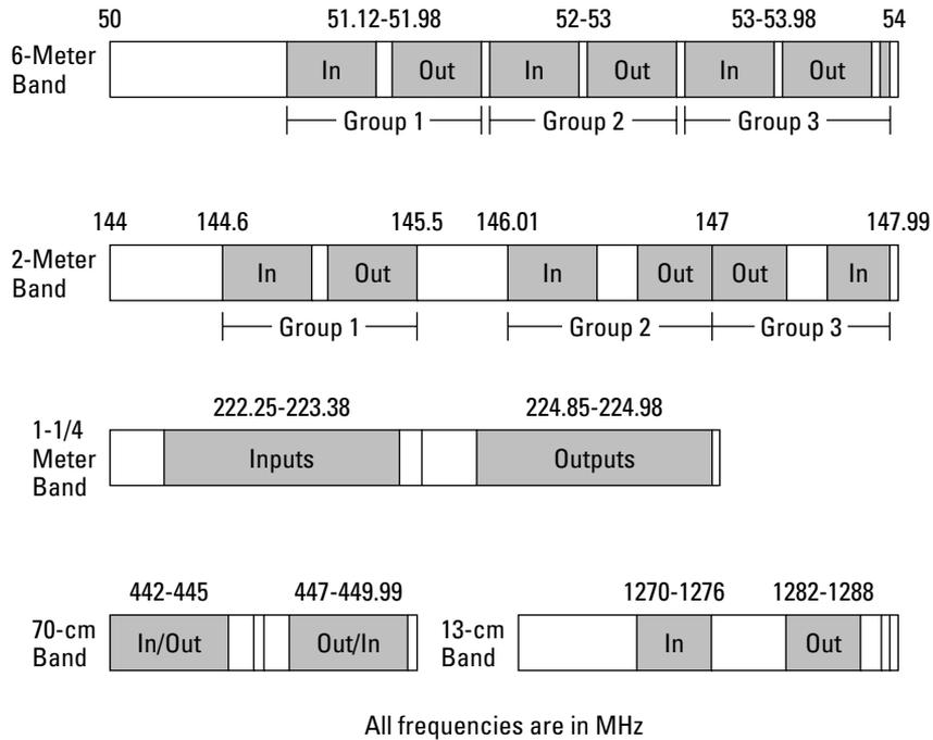
**Figure 9-3:** Repeater allocations on the five primary VHF/UHF bands.
